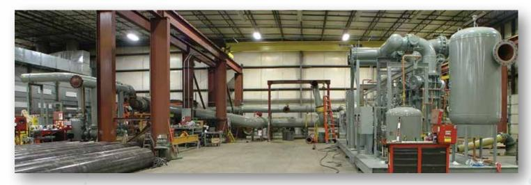
Our flow test stand can test up to 30,000 GPM, ensuring every Systecon system is tested to full design flow - something that field built systems can't always accommodate.
