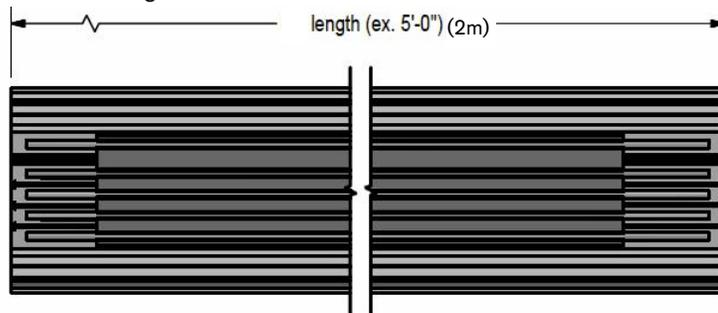
**Step 2.** Cut the housing/insulator to required length. \*\*\*(Be sure to clean all parts of metal and plastic shavings after cuts.)\*\*\*
