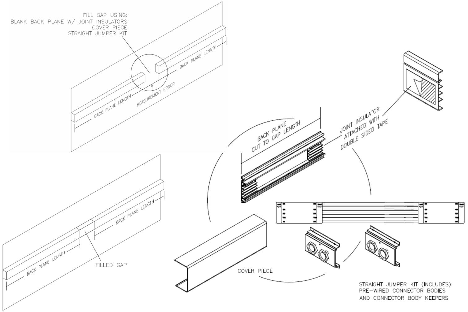
The straight jumper kits (and the elbow sections) include all the necessary parts to jump between the two backplanes. Installation of the straight jumper is similar to how the field modified elbows are installed.
