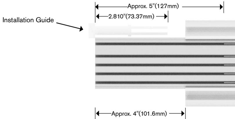
**Step 5.** Copper adjustment. Using the provided guide, slide the copper back into position. The field tool will properly align the copper in the insulator as shown below. Repeat until all conductors are in position.
