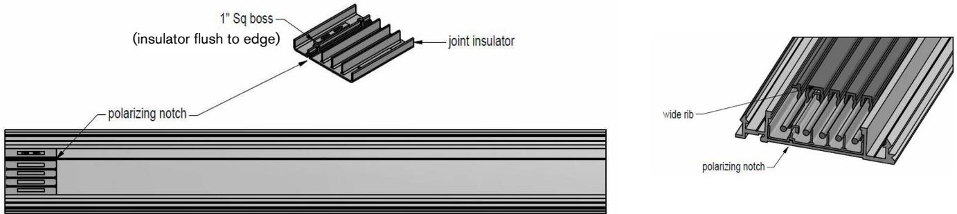
**Step 8.** Dry fit the other joint insulator, make sure that it slides under the insulator. (It should be flush with the end of the backplane housing.) Now remove the joint insulator, apply glue and reinsert it back on the backplane. Let it dry.
