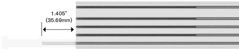
**Step 6.** Install the joint insulator by super gluing it to one end of the backplane. Let it dry. (The housing should have nothing protruding.) Be aware of the polarizing notch on the backplane and the joint insulator.
